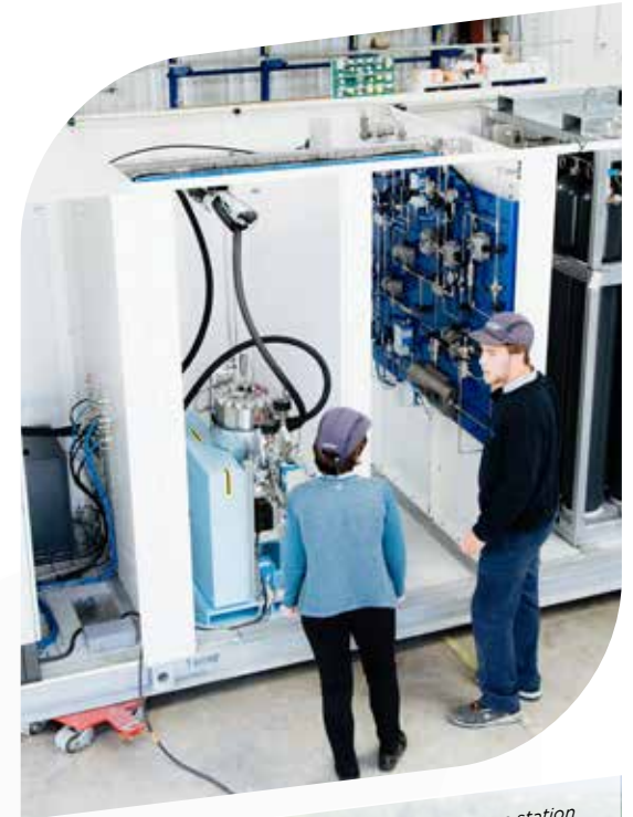
R-Hynoca project in Strasbourg | Dual pressure station (350 and 700 bar), distribution capacity of 700 kg / day (equivalent to a fleet of 30 buses, or 70 light commercial vehicles, or 150 vehicles), associated with a hydrogen tube trailers refill point. Client: R-GDS. This project received a funding from the FCH-JU, with the support of the Horizon 2020 research and innovation program of the European Union, Hydrogen Europe and Hydrogen Europe Research.
