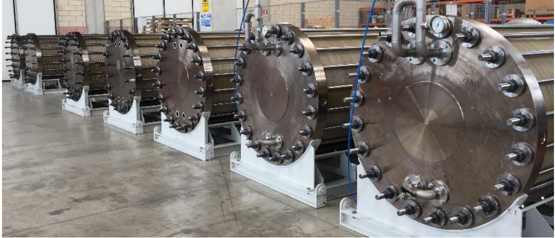
4 MW of electrolysis capacity for a Power to Gas project in the Hebei province, China
