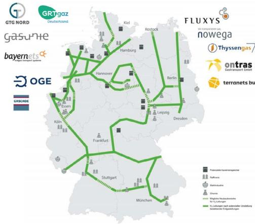
11 German TSO published a hydrogen strategy for the conversion of existing pipelines into a H2 backbone. It encompasses 5.900 km of pipeline of which 90 % are existing natural gas pipes. This hydrogen grid connects industrial clusters, fuelling stations for mobility on land and water as well as distribution grids. The TSO are actively working on technical solutions and the details of the grid planning.
