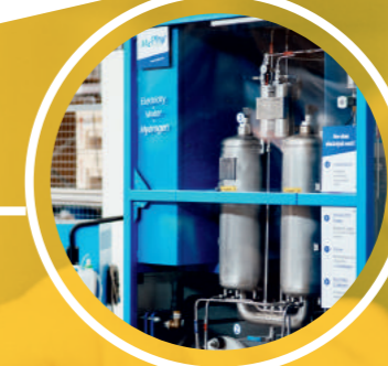
McLyzer Electrolyzers From 10 to 800 Nm 3 /h in series 10 to 30 bar
