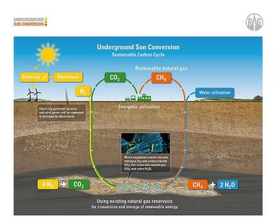
RAG has developed an innovative approach to produce and store green methane from hydrogen generated by renewable energies and microbacteria. The synthetic natural gas will be produced and stored directly in a natural gas reservoir more than 1,000 m underground, then fed into the pipeline network to be delivered on demand to consumers.
